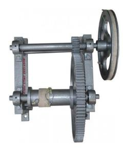
Apparatus consists of a heavy duty C.I. wall brackets. The grooved wheel is of 25 cm dia, and a set of gearing arrangements (machine cut gears) are provided for measurement of efficiency of winch crab.
